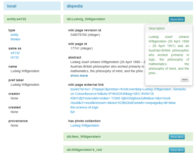
Figure 4: Screenshot of the linking interface listing the linking candidates for the InPhO entity “Ludwig Wittgenstein.” The link candidate ranking on the right is influenced by the lexical similarity and the semantics of the source entity. Users can easily identify the correct linking candidate by browsing its semantic properties and Wikipedia abstract.
